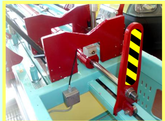
Closing cylinder of pneumatic type (for plunger cylinders) with stroke gauging system. OPTTT000021
