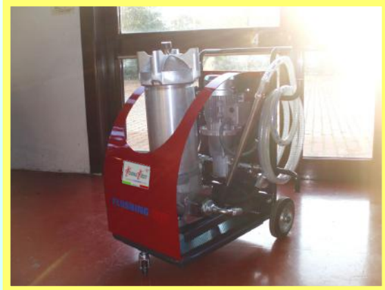
Mobile electro-pump unit with 10 µ filter. ATZTT0000001
