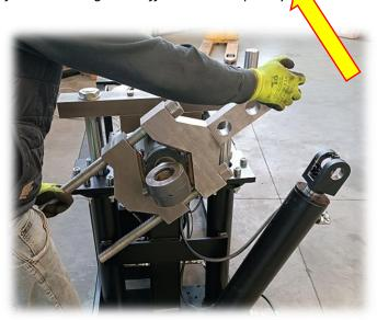
Once the release cylinder has been disconnected, the operator will have complete freedom to rotate the key manually to unscrew the head:
