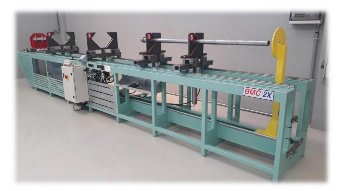
Machine equipped for complete support of the components being processed, with a self-centering system for inserting the stem:
